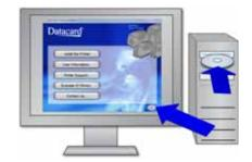
3 Connect the printer to the PC using the USB data cable. Position the USB cable at an angle to properly insert it into the printer.
